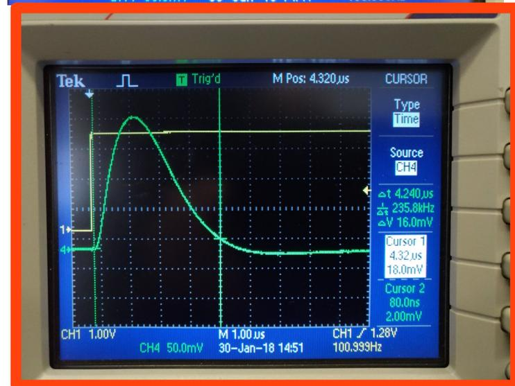
Parameters adjusted via repeater. Improving the signal shape is useful to prevent pile up
