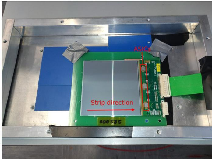
Each detector is made of double-side microstrip planes (XY or UV).
