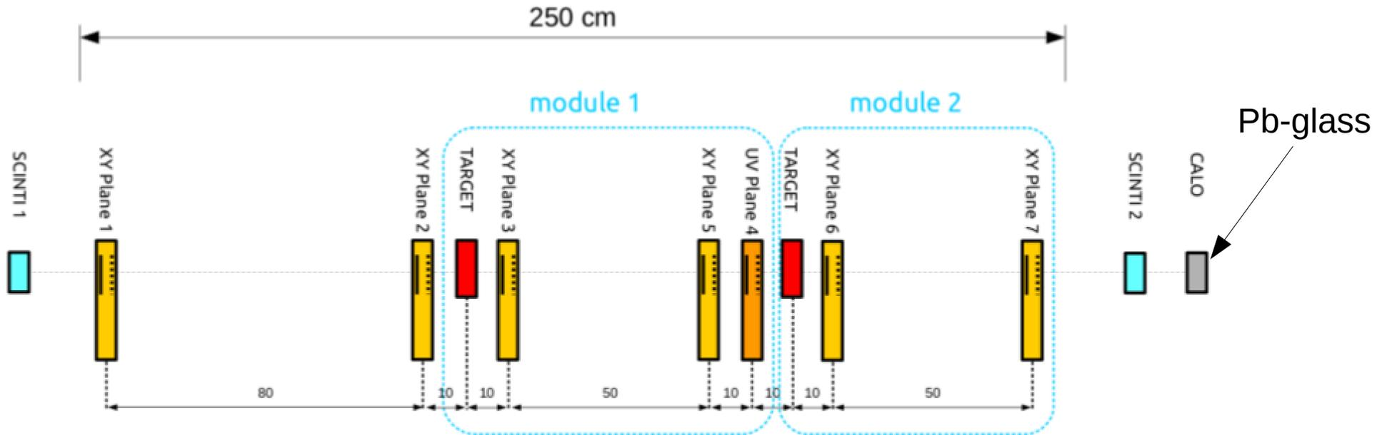
Scintillators: 2  $100 \times 100 \text{ mm}^2$
