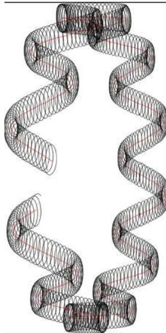
Electrons of  $\sim 30$  keV from a gaseous source were let to decay within a 1 tesla field with an additional pair of coils to set up a *magnetic trap*:
