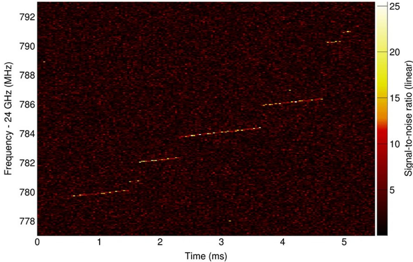
Power from a single electron orbiting in a magnetic field versus time and the frequency of the electron's orbit. The straight streaks correspond to the electron losing energy (and orbiting faster) as it radiates. The jumps correspond to the loss of energy when the electron collides with an atom or molecule. [Asner et al. [PRL **114**, 162501]
