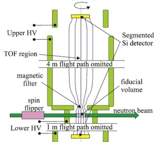
Figure 9. Principle of the Nab spectrometer in the vertical orientation. Magnetic field lines (shown in blue) electrodes (light green boxes), and coils (not shown) possess cylindrical symmetry around the vertical axis. The neutron beam is unpolarized for Nab, but can be polarized for later experiments.
