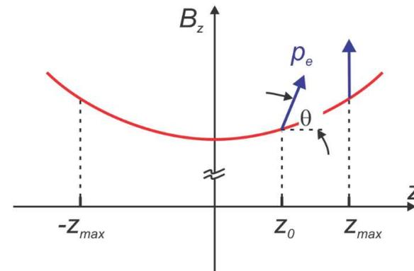
Longitudinal comp. of momentum decreases as  $B$  increases up to return point,  $z_{max}$ . Axial oscillations with  $\omega_z$ .
