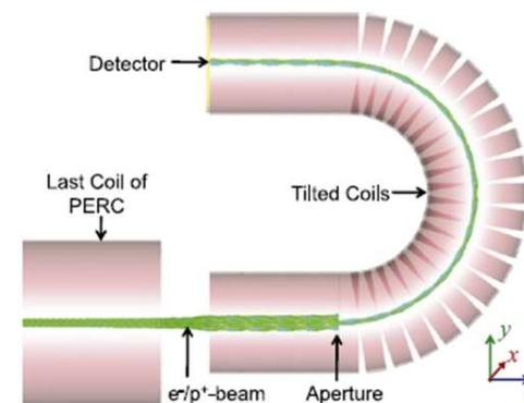
Fig. 5. The design of the  $R \times B$  drift spectrometer at the end of PERC, and the simulated trajectories of  $e^-/p^+$ .
