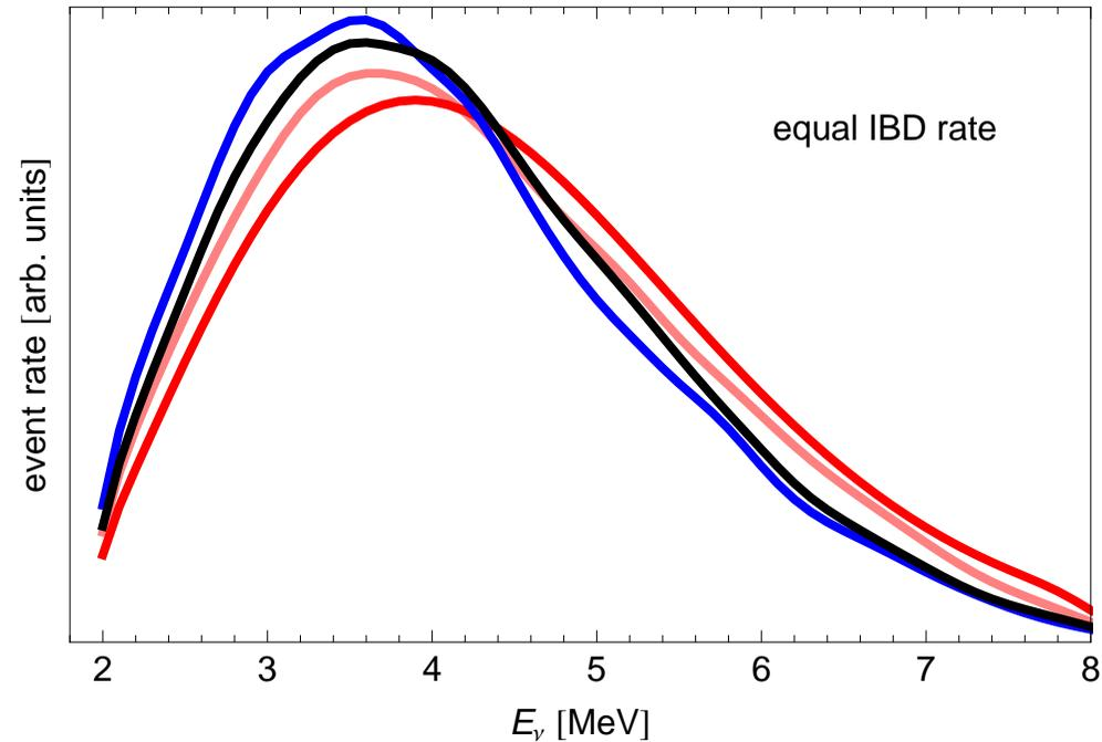
Pu239 has a softer neutrino spectrum than U235 – as a consequence the neutrino spectrum becomes softer for higher burn-up
