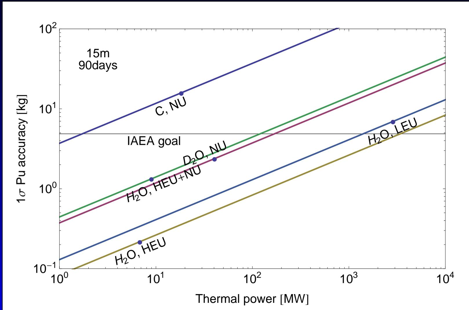
Standard detector – based on detailed SCALE calculations.
