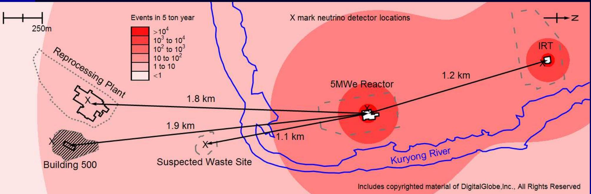
The IRT is a small (6MWth) HEU reactor which has been under safeguards since 1977, neutrinos from the 5MWe will be visible at its site
