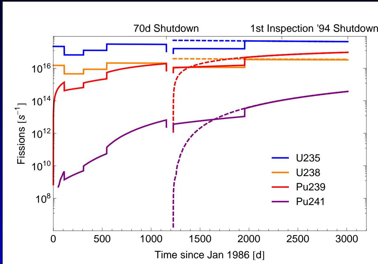
Based on a full SCALE calculation using a detailed power history and the magnox cross section libraries.
